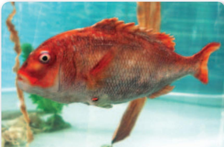
■ **Figure 6.6** Scientists developing submarine technology created a robot that looks and swims like a real fish. Its body is made of a silicon resin that softens in water.
