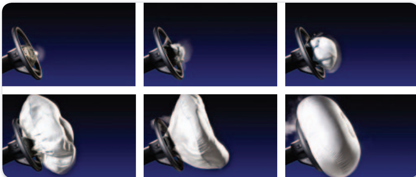
■ Figure 9.11 The decomposition of sodium azide, which produces a gas, is the chemical reaction that inflates air bags.
