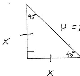
$$\begin{aligned} x^2 + x^2 &= H^2 \\ H &= x\sqrt{2} \quad \sqrt{2x^2} = \sqrt{H^2} \\ H &= x\sqrt{2} \end{aligned}$$
