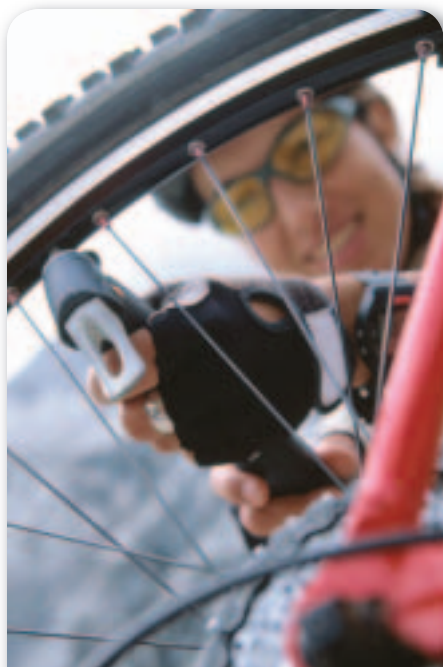
■ Figure 13.6 The volume and temperature of this tire stay the same as air is added. However, the pressure in the tire increases as the amount of air present increases.
