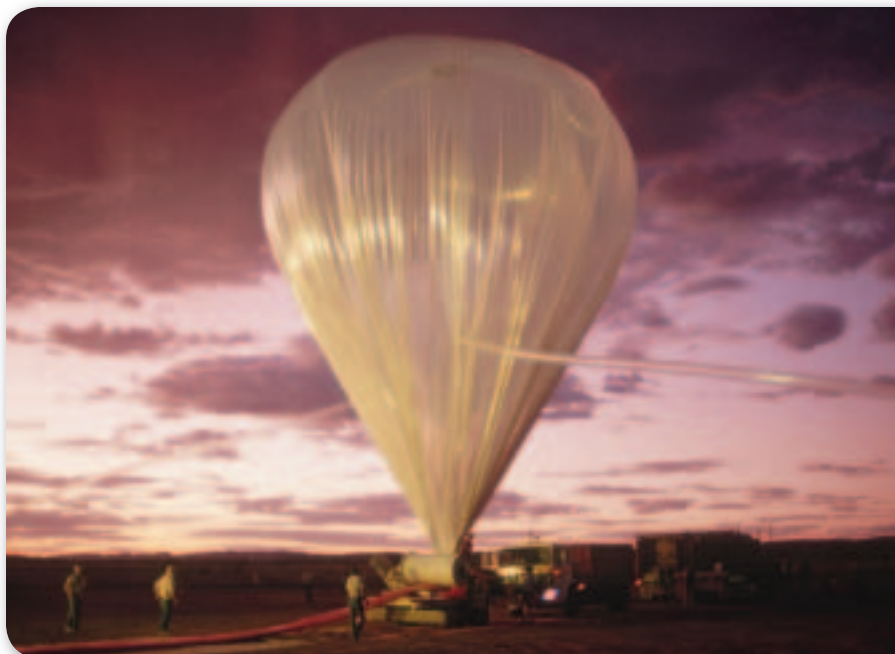
■ Figure 13.4 Tethers attached at the sides of a weather balloon hold it in place while it is being filled with helium or hydrogen gas. Weather balloons carry instruments that send data, such as air temperature, pressure, and humidity, to receivers on the ground. As the balloon rises, its volume responds to changes in temperature and pressure, expanding until the sides burst. A small parachute returns the instruments to Earth.
