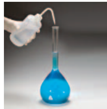
Step 3: Distilled water is added to the flask to bring the solution level up to the calibration mark.
