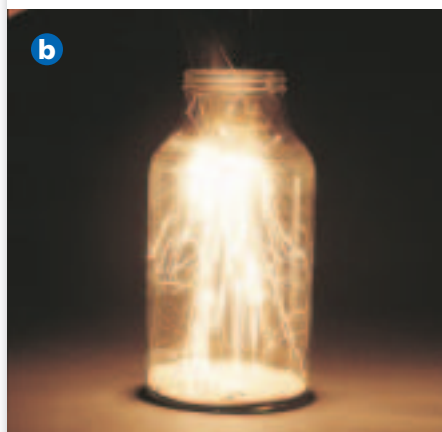
■ Figure 16.10 The greater surface area of the steel wool means that more collisions can occur between the metal and oxygen.
