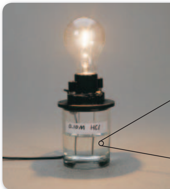
■ Figure 18.11 The light glows brightly when electrodes are placed in 0.10M hydrochloric acid solution because all of the HCl is in the form of hydronium ions and chloride ions.
