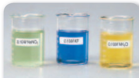
■ Figure 18.26 The indicator bromthymol blue provides surprising results when added to three solutions of ionic salts. An \text{NH}_4\text{Cl} solution is acidic, a \text{NaNO}_3 solution is neutral, and a \text{KF} solution is basic. The explanation has to do with the strengths of the acid and base from which each salt was formed.
