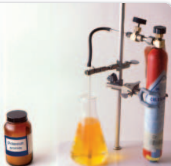
■ Figure 19.2 The reaction between aqueous bromide ions and chlorine gas is a redox reaction. Here, electrons are transferred from bromide ions to chlorine.
