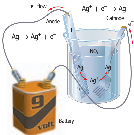
■ Figure 20.23 Power is needed to oxidize silver at the anode and reduce silver at the cathode. In an electrolytic cell used for silver plating, the object to be plated is the cathode where silver ions in the electrolyte solution are reduced to silver metal and deposited on the object.
