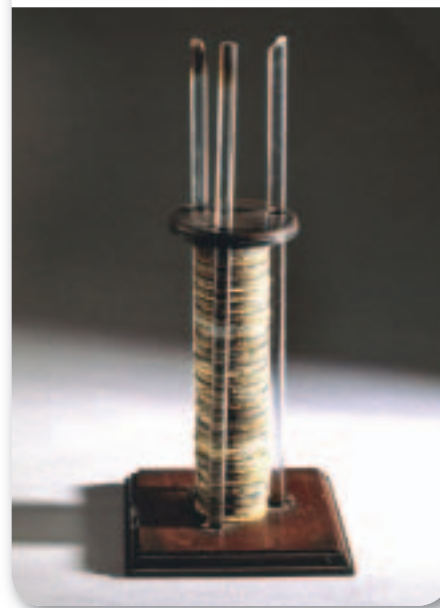
■ Figure 20.3 This replica of one of Alessandro Volta's first cells consists of discs of zinc and copper arranged in alternating layers and separated by cloth or cardboard soaked in an acidic solution. Electric current increased with the number of metal discs used.
