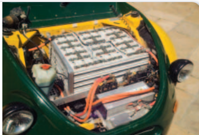
Lithium battery packs power this experimental car to a maximum speed of 113 km/h. The car has a range of over 320 km.
