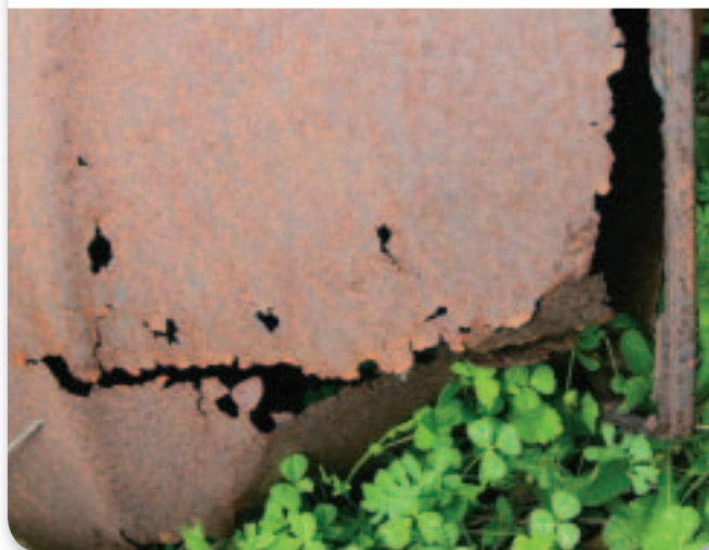
■ Figure 20.14 Left unattended in the presence of air and moisture, this iron barrel is slowly being oxidized to rust ( \text{Fe}_2\text{O}_3 ).
