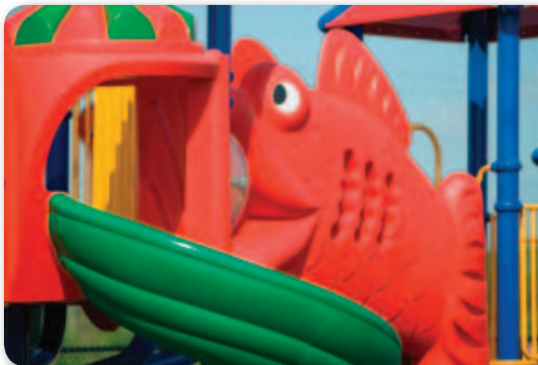
■ Figure 22.14 Low density polyethylene (LDPE) is made from gaseous ethene under high pressure in the presence of a catalyst. LDPE is used for playground equipment because it is easy to mold into various shapes, it is easy to dye into many colors, and it is durable.
