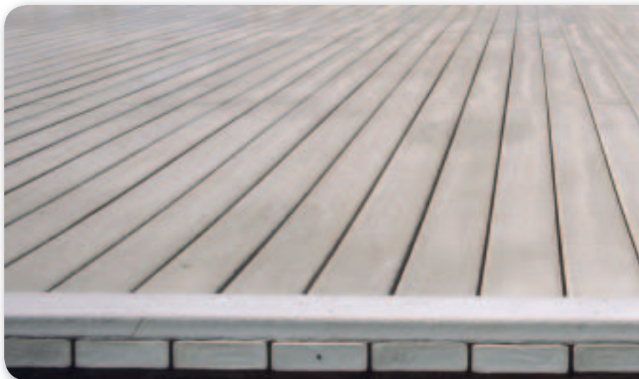
■ Figure 22.20 Plastic lumber is made from recycled plastic, such as used soft-drink bottles, milk jugs, and other polyethylene waste.
