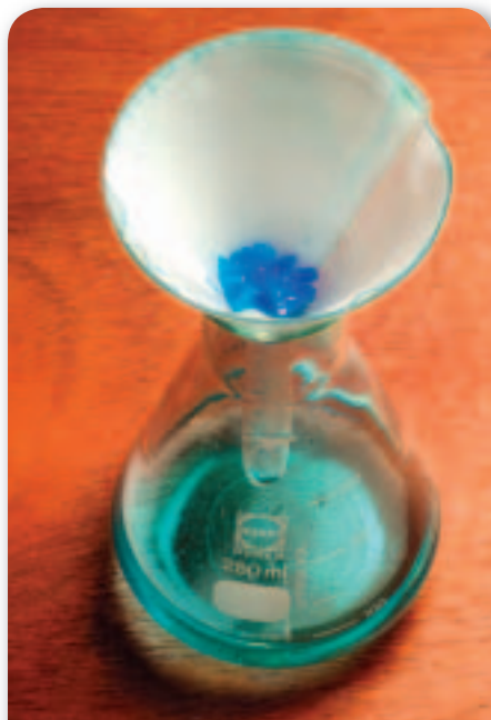
■ Figure 3.13 As the mixture passes through the filter, the solids remain in the filter, while the filtrate (the remaining liquid) is collected in the beaker.
