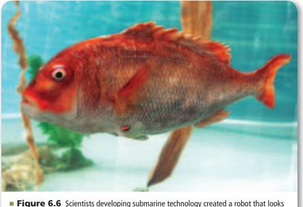
and swims like a real fish. Its body is made of a silicon resin that softens in water.
