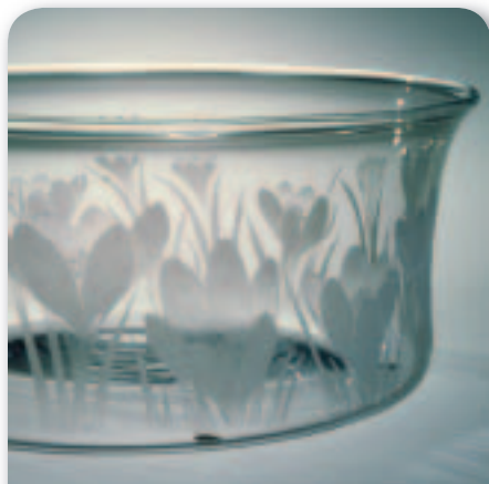
■ Figure 8.6 The frosted-looking portions of this glass were chemically etched using hydrogen fluoride (HF), a weak acid. Hydrogen fluoride reacts with silica, the major component of glass, and forms gaseous silicon tetrafluoride ( \text{SiF}_4 ) and water.
